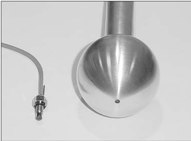
Fig. 4 Modified COTS pressure transducer and the spherical probe head.
